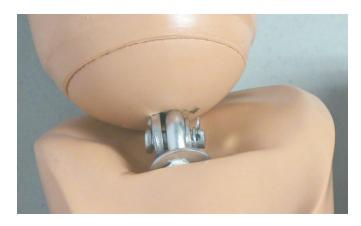
6. Install the washer and the spring clip on the clevis pin
