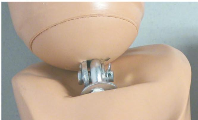
6. Install the washer and the spring clip on the clevis pin
