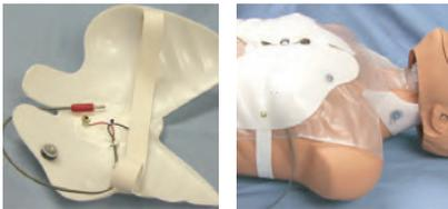
The switch that connects the blue light terminals lies on the sternum of the chest plate. If your correct hand position does not turn on the light, check to see that the switch strip is positioned in line with the sternum. If it twists off center, it will not make contact when hands are placed upon it. If the blue light is constantly on, lightly bend the strip ends up so that they don't contact the terminals until hand pressure is applied. If your airway disconnects from
