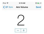
**Arm Volume**: On the main screen click on the blue arrow on the right side of the screen next to the Arm Volume, this will open up the Arm Volume Screen. Change the values by tapping on the + and/or – symbols.
