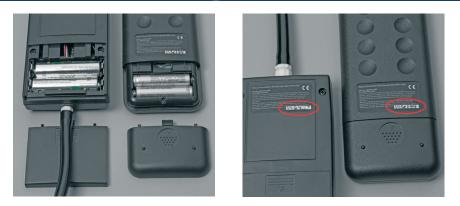
When paring to use your SmartScope<sup>™</sup>and remote, use batteries that are fully charged and positioned correctly. The SmartScope<sup>™</sup> is not equipped with a power button, this may drain the useful life of your batteries.
